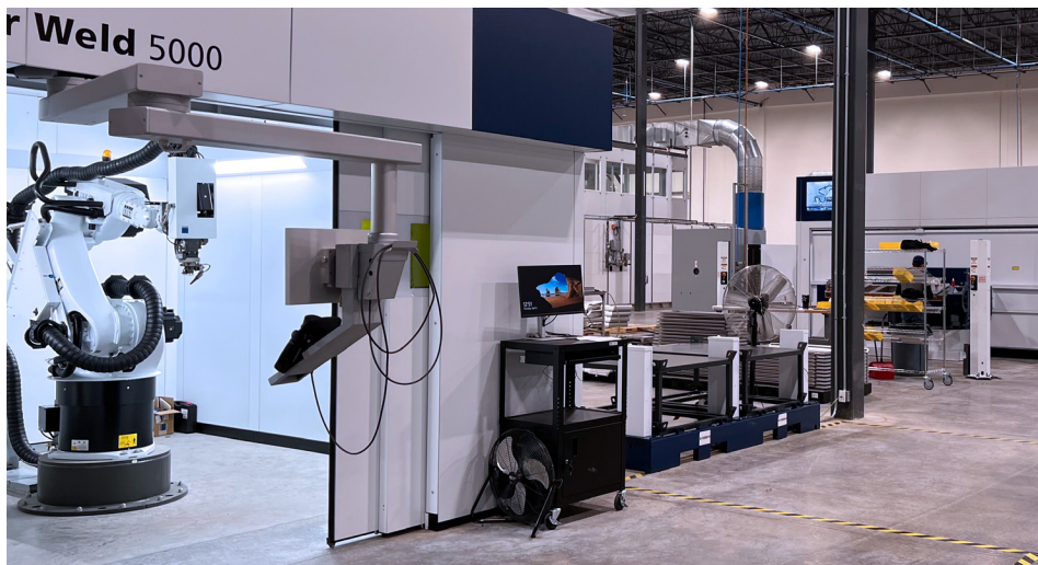
Robotic welders and automated lasers are two of the many tools used by SmartCap to build their various truck cap designs. They all run on the Internet of Things (IoT). This requires special bandwidth channeled via WiFi from the central Managed Network Edge platform.
