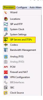
This will bring up the SIP and ITSP configuration screen. It has three tabs along the top. To configure the SIP server, click on the SIP tab. For ITSPs, click on the ITSP tab. To set up the authentications, click on the last tab, Authentication.
